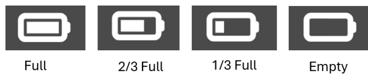
Figure: Battery level indicator for monitoring devices that provide battery level information (i.e. telemetry devices).
